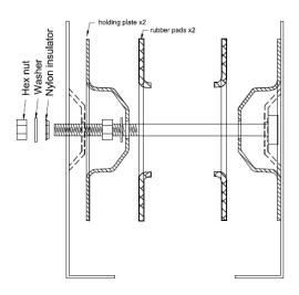
CL-500D includes 2 L bracket, 2 holding plates, 2 rubber pads, bolt, 2 hex nuts, 3 washers, insulator and spring washer.
