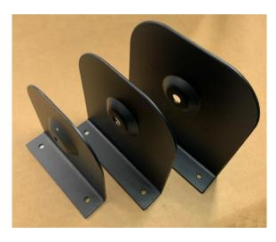
This CL toroidal transformer vertical mount brackets are built for strength and durability, using 0.08" thick steel to provide a solid support system. They are designed to work with many different transformer makes and models, ranging from 50VA to 800VA. This bracket offers three sizes for customers to choose from, ensuring a perfect fit for their needs. The vertical mounting feature not only keeps the transformer secure but also makes the setup safe and reliable.
