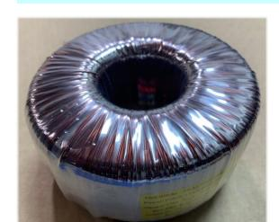
The 700VA industrial toroidal power transformer has higher efficiency than EI transformers, typically around 95 to 99%. Because of the effective containment of the magnetic flux inside the core, toroidal transformer will have a lot less interference with adjacent components. It has very lower mechanical humming and lower heat generated.
