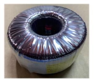
The 700VA industrial toroidal power transformer has higher efficiency than EI transformers, typically around 95 to 99%. Because of the effective containment of the magnetic flux inside the core, toroidal transformer will have a lot less interference with adjacent components. It has very lower mechanical humming and lower heat generated.
