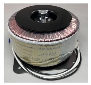
The 500VA industrial toroidal power transformer offers higher efficiency than EI transformers, typically ranging up to 97%. Due to its effective containment of magnetic flux within the core, it significantly reduces interference with nearby components. Additionally, it generates a lot less mechanical humming and heat.
