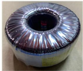
The 500VA industrial toroidal power transformer has higher efficiency than EI transformers, typically around 95 to 99%. Because of the effective containment of the magnetic flux inside the core, toroidal transformer will have a lot less interference with adjacent components. It has very lower mechanical humming and lower heat generated.
