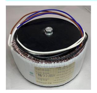
The 4000VA industrial toroidal power transformer offers higher efficiency than EI transformers, typically ranging up to 97%. Due to its effective containment of magnetic flux within the core, it significantly reduces interference with nearby components. Additionally, it generates a lot less mechanical humming and heat.
