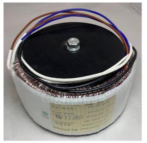
The 2000VA industrial toroidal power transformer offers higher efficiency than EI transformers, typically ranging up to 97%. Due to its effective containment of magnetic flux within the core, it significantly reduces interference with nearby components. Additionally, it generates a lot less mechanical humming and heat.
