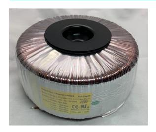
The 1300VA industrial toroidal power transformer has higher efficiency than EI transformers, typically around 95 to 99%. Because of the effective containment of the magnetic flux inside the core, toroidal transformer will have a lot less interference with adjacent components. It has very lower mechanical humming and lower heat generated.
