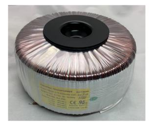
The 1300VA industrial toroidal power transformer has higher efficiency than EI transformers, typically around 95 to 99%. Because of the effective containment of the magnetic flux inside the core, toroidal transformer will have a lot less interference with adjacent components. It has very lower mechanical humming and lower heat generated.
