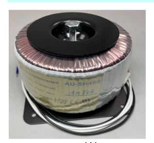
The 1000VA industrial toroidal power transformer offers higher efficiency than EI transformers, typically ranging up to 97%. Due to its effective containment of magnetic flux within the core, it significantly reduces interference with nearby components. Additionally, it generates a lot less mechanical humming and heat.
