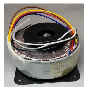
The 1000VA industrial toroidal power transformer offers higher efficiency than EI transformers, typically ranging up to 97%. Due to its effective containment of magnetic flux within the core, it significantly reduces interference with nearby components. Additionally, it generates a lot less mechanical humming and heat.
