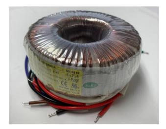
The 25VA industrial toroidal power transformer has higher efficiency than EI transformers, typically around 95 to 99%. Because of the effective containment of the magnetic flux inside the core, toroidal transformer will have a lot less interference with adjacent components. It has very lower mechanical humming and lower heat generated.
