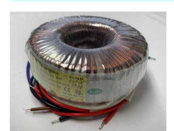
The 25VA industrial toroidal power transformer has higher efficiency than EI transformers, typically around 95 to 99%. Because of the effective containment of the magnetic flux inside the core, toroidal transformer will have a lot less interference with adjacent components. It has very lower mechanical humming and lower heat generated.
